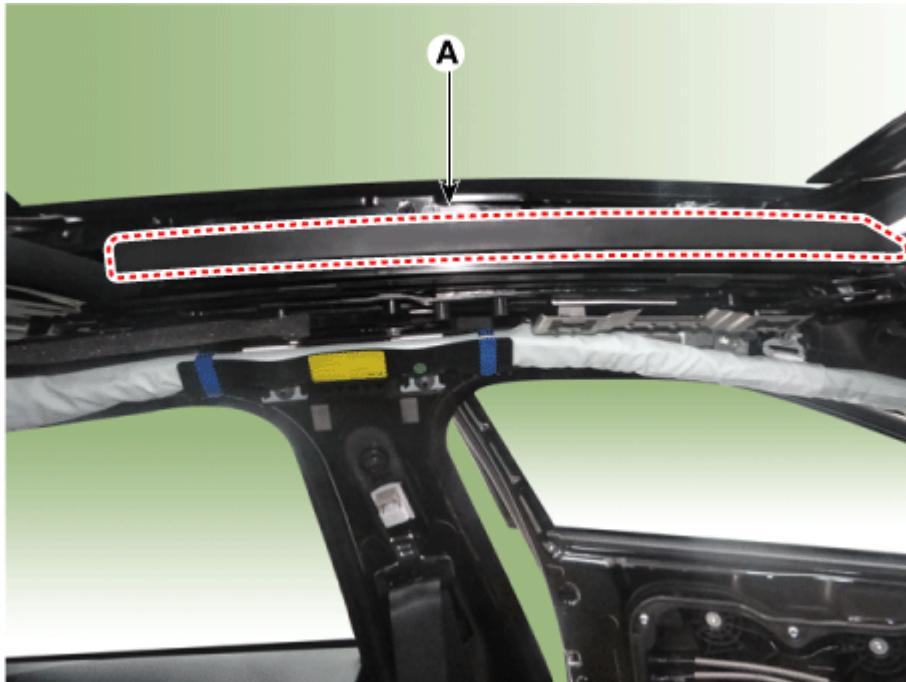
3. Loosen the mounting screws (A) on both sides.
