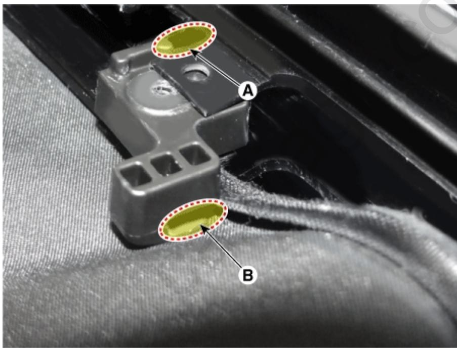
9. Loosen the roller blind shoe clip mounting screw (A).
