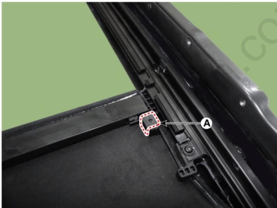
11. Remove roller blind bar (B) by pressing locking pin (A) with using flat-tip screwdriver.
