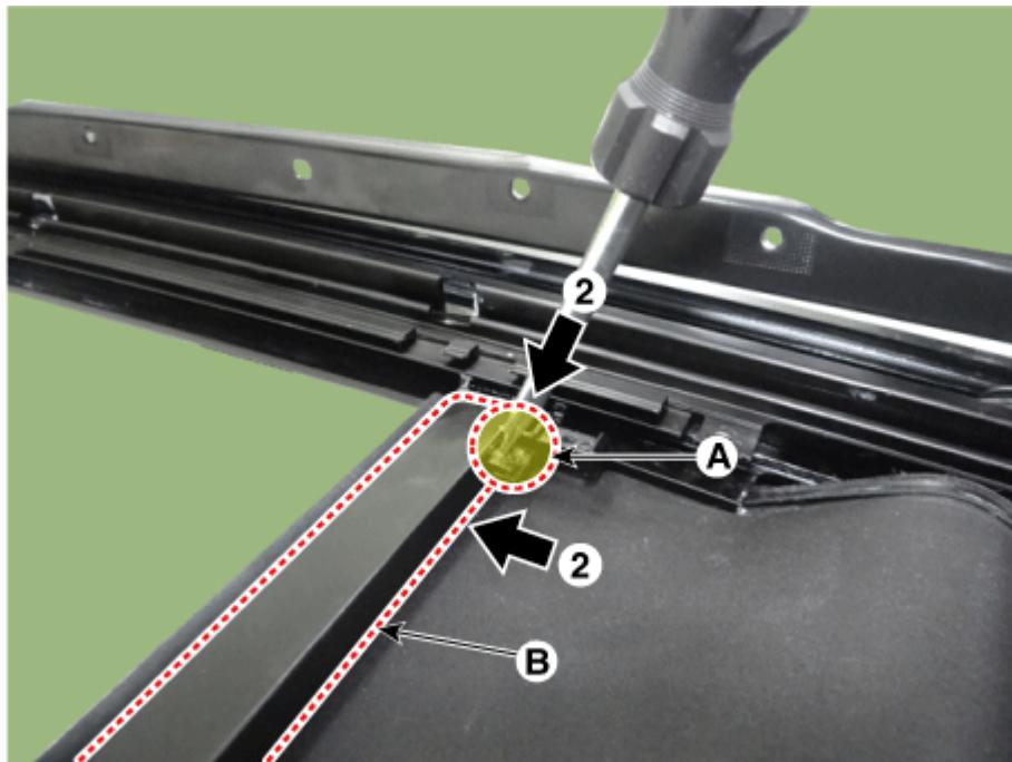
12. Separate right side of the roller blind (A) by pushing washer (B).
